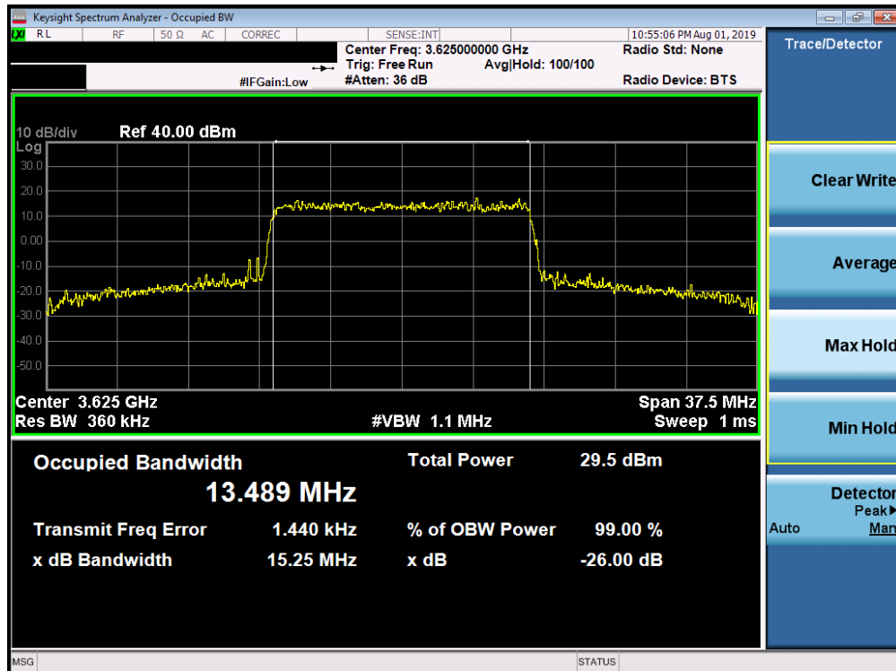
Plot 7-8. Occupied Bandwidth Plot (Band 48 - 15.0MHz 16-QAM - Full RB Configuration)
