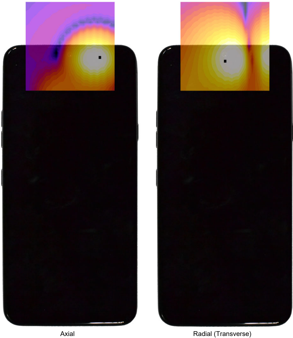
Figure 16-3 T-Coil Scan Overlay Magnetic Field Distributions
