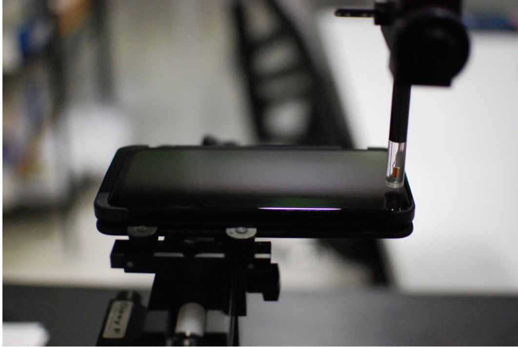
Figure 16-5 Test Setup for Wireless Device with Dual Display – Open
