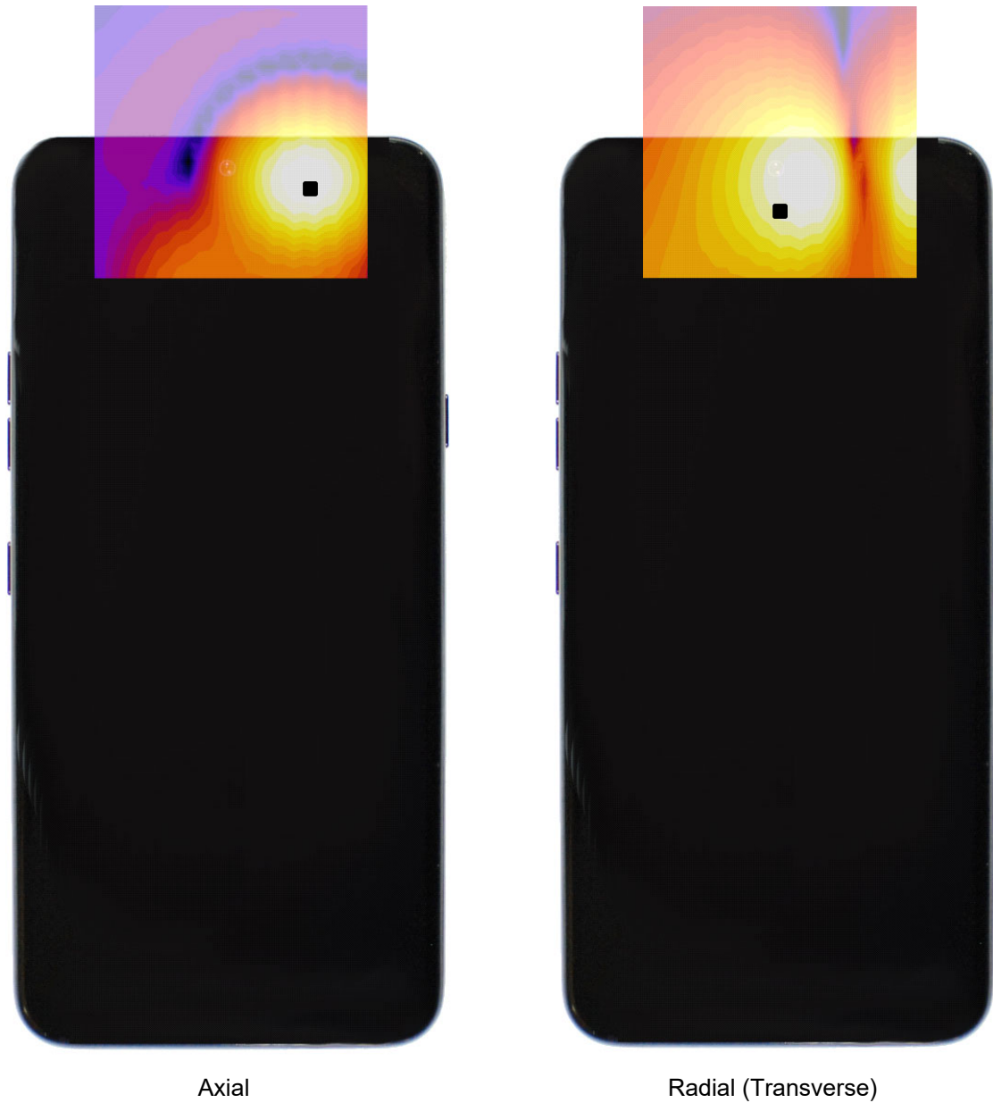
Figure 16-7 T-Coil Scan Overlay Magnetic Field Distributions
