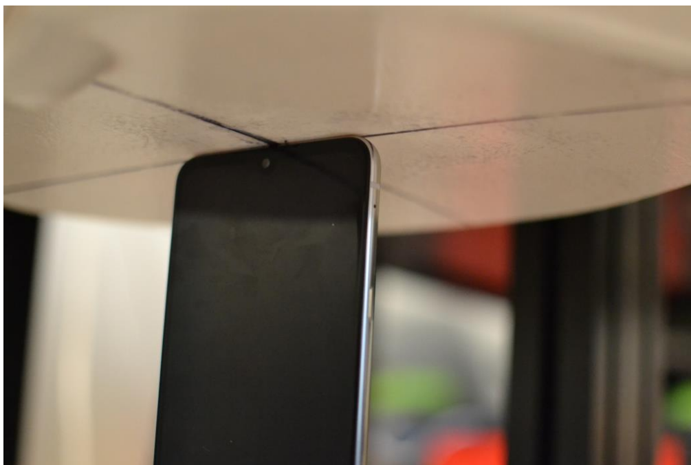
SAR Test Setup Photo 11 – Top Side at 0 mm
