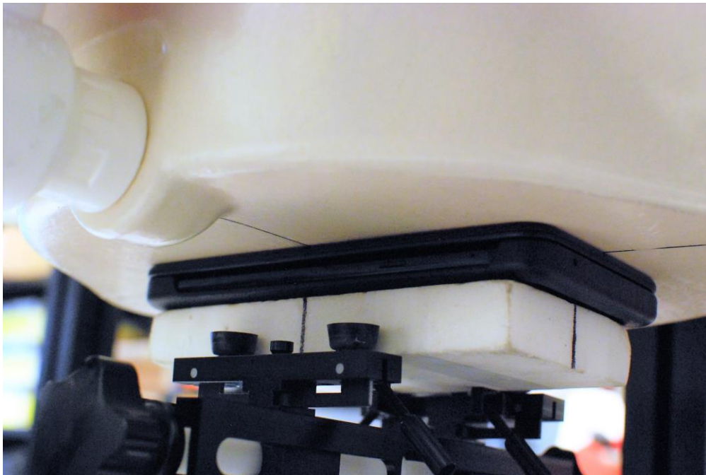
SAR Test Setup Photo 22 – Front Side at 0 mm with Dual Display Cover Position #1 (0 degrees)
