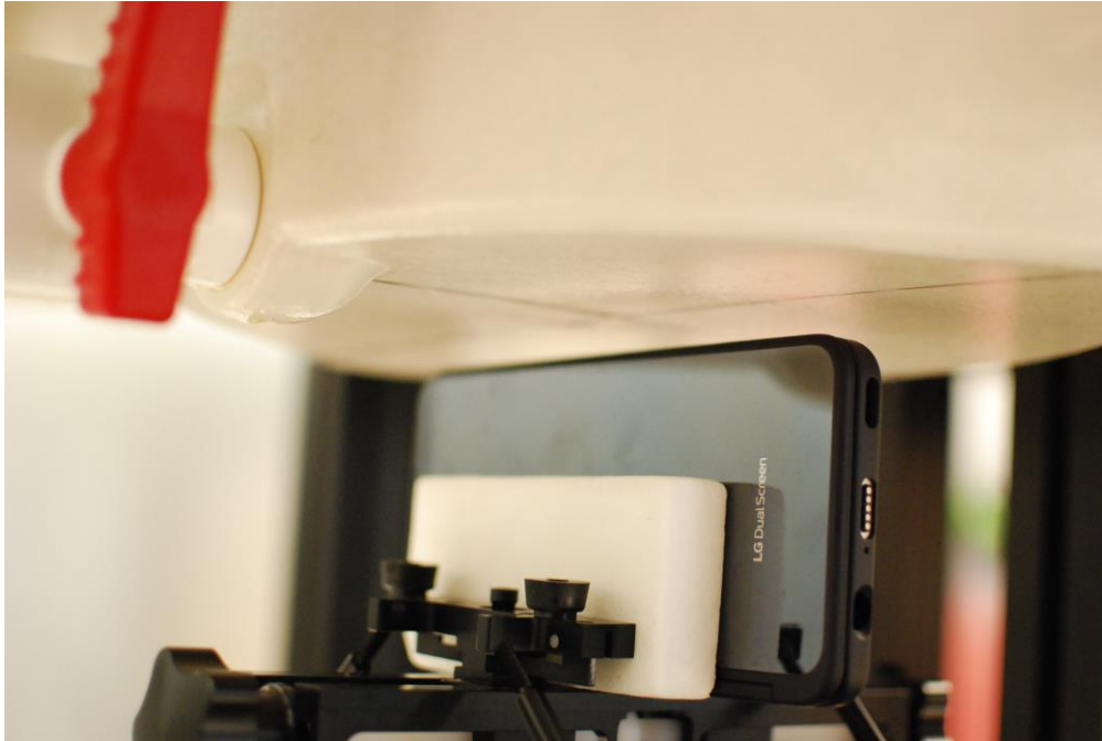
SAR Test Setup Photo 37 – Right Side at 10 mm with Dual Display Cover Position #1 (0 degrees)
