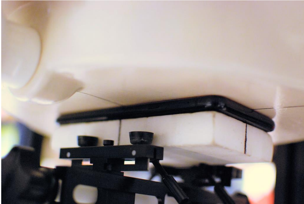
SAR Test Setup Photo 21 – Front Side at 0 mm
