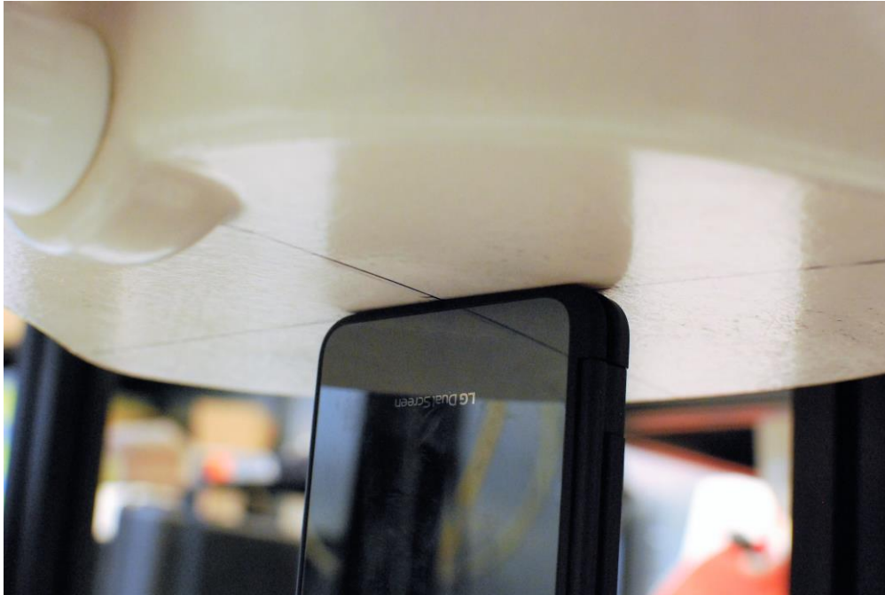
SAR Test Setup Photo 33 – Bottom Side at 0 mm with Dual Display Cover Position #1 (0 degrees)
