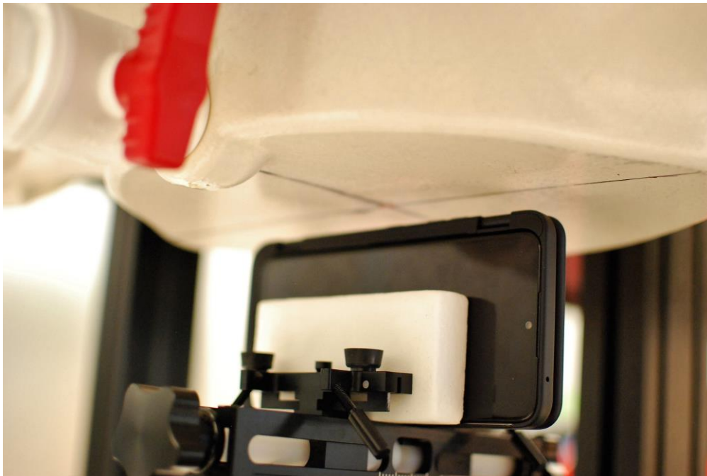
SAR Test Setup Photo 42 – Left Side at 10 mm with Dual Display Cover Position #3 (360 degrees)
