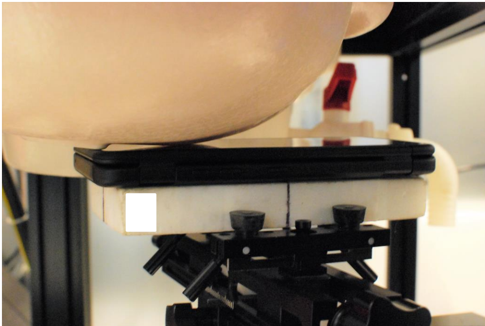
SAR Test Setup Photo 2 – Right Cheek with Dual Display Cover Position #1 (0 degrees)
