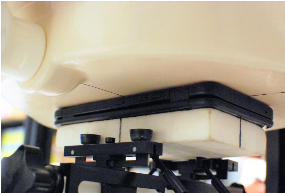
SAR Test Setup Photo 16 – Back Side at 0 mm with Dual Display Cover Position #1 (0 degrees)
