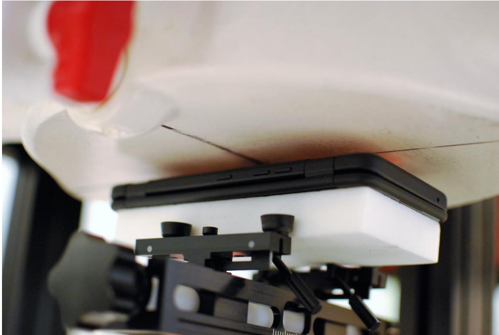
SAR Test Setup Photo 11 – Back Side at 10 mm with Dual Display Cover Position #1 (0 degrees)
