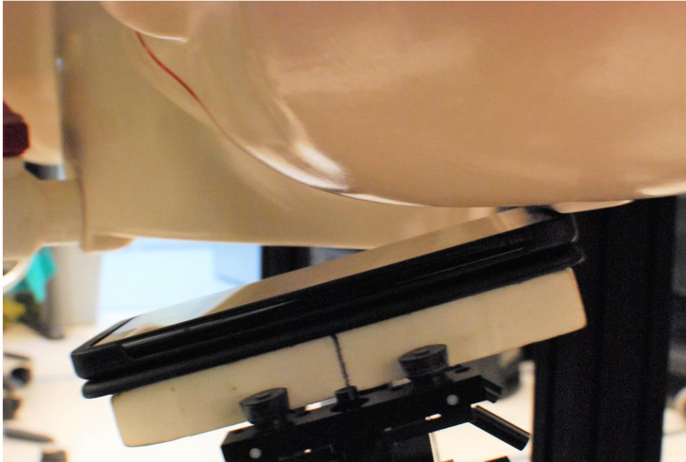
SAR Test Setup Photo 9 – Left Tilt with Dual Display Cover Position #3 (360 degrees)
