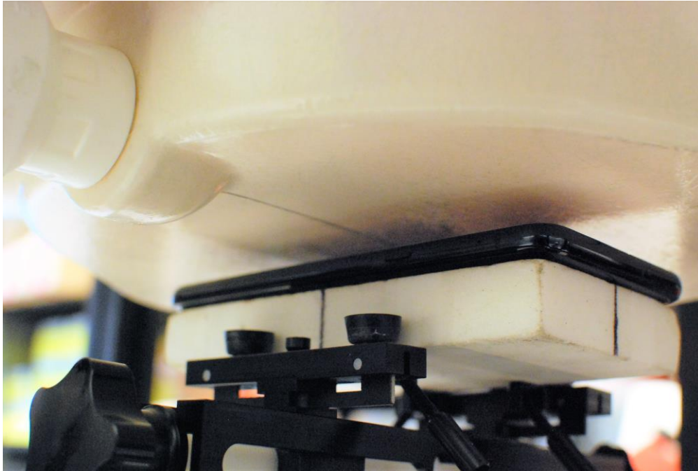
SAR Test Setup Photo 19 – Front Side at 10 mm
