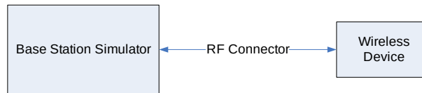
Figure 9-4 Power Measurement Setup
