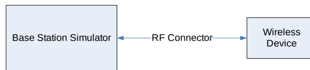
Figure 9-3 Power Measurement Setup
