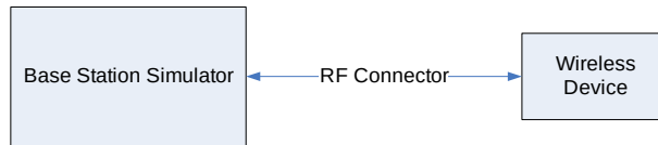
Figure 9-2 Power Measurement Setup
