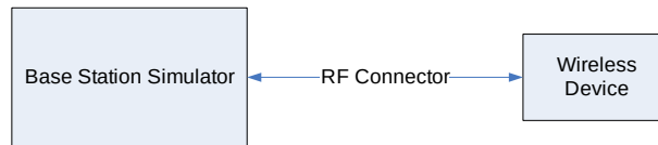
Figure 9-4 Power Measurement Setup
