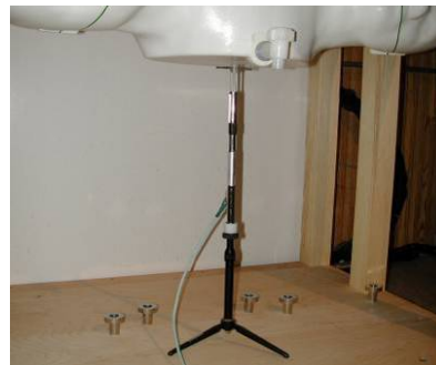
Figure 10-2 System Verification Setup Photo
