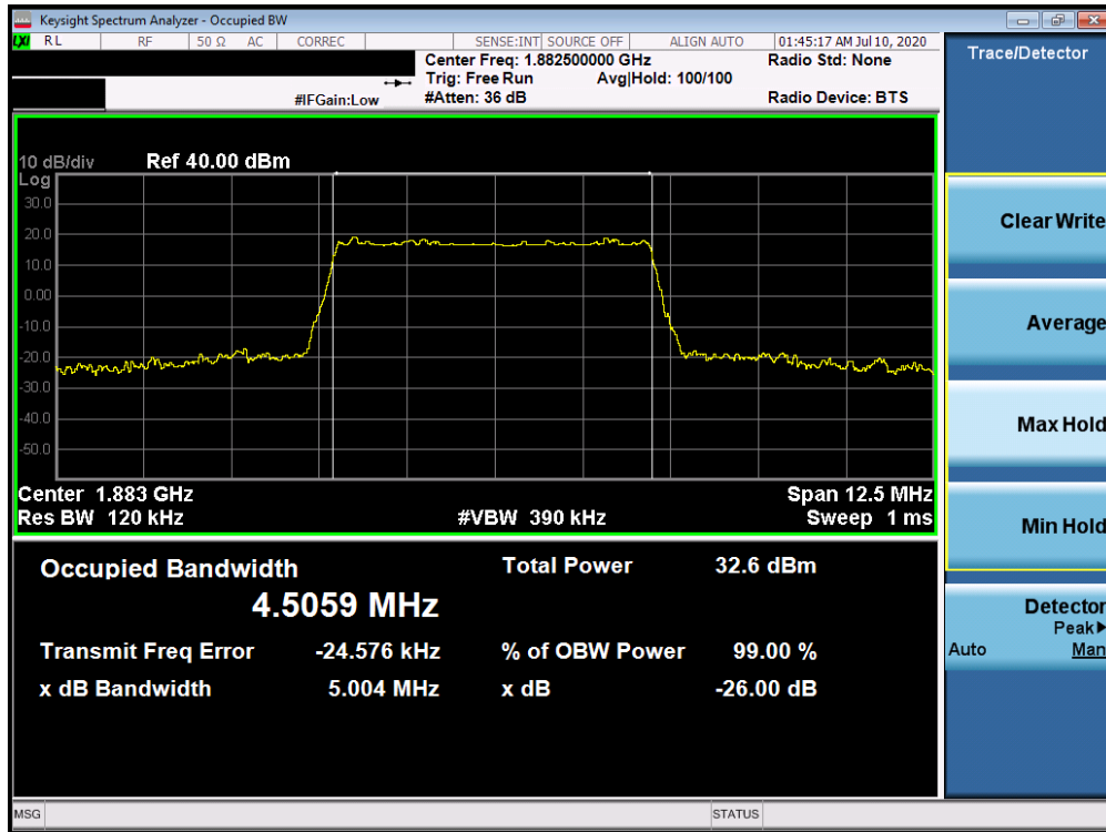
Plot 7-134. Occupied Bandwidth Plot (Band 25/2 - 5.0MHz QPSK - Full RB Configuration)
