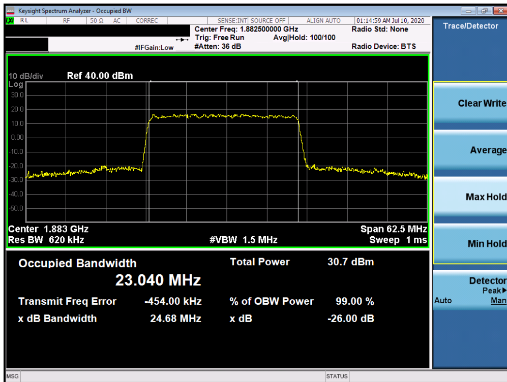
Plot 7-169. Occupied Bandwidth Plot (n25 25MHz 64QAM-CP-OFDM- Full RB Configuration)
