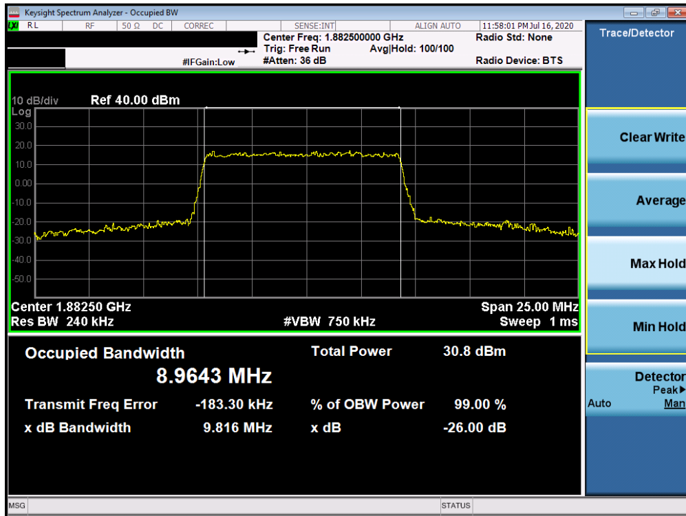
Plot 7-187. Occupied Bandwidth Plot (n25 10MHz QPSK-CP-OFDM - Full RB Configuration)
