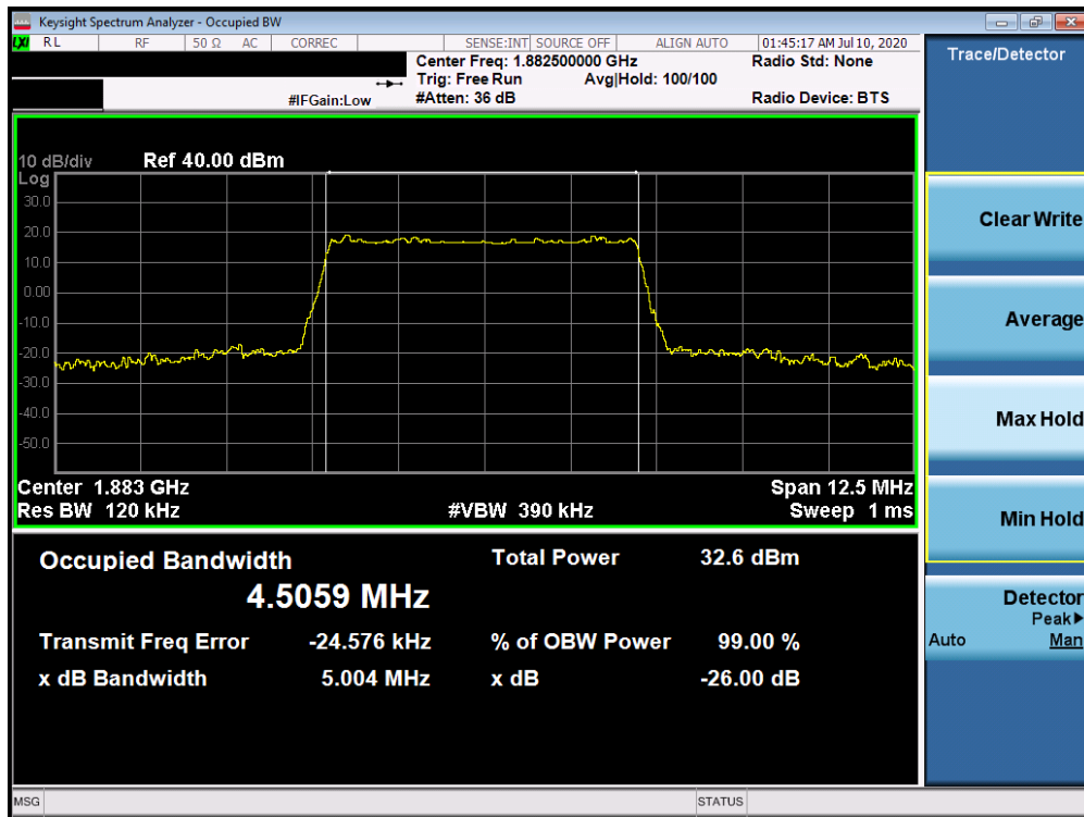
Plot 7-147. Occupied Bandwidth Plot (n25 5MHz QPSK-CP-OFDM - Full RB Configuration)
