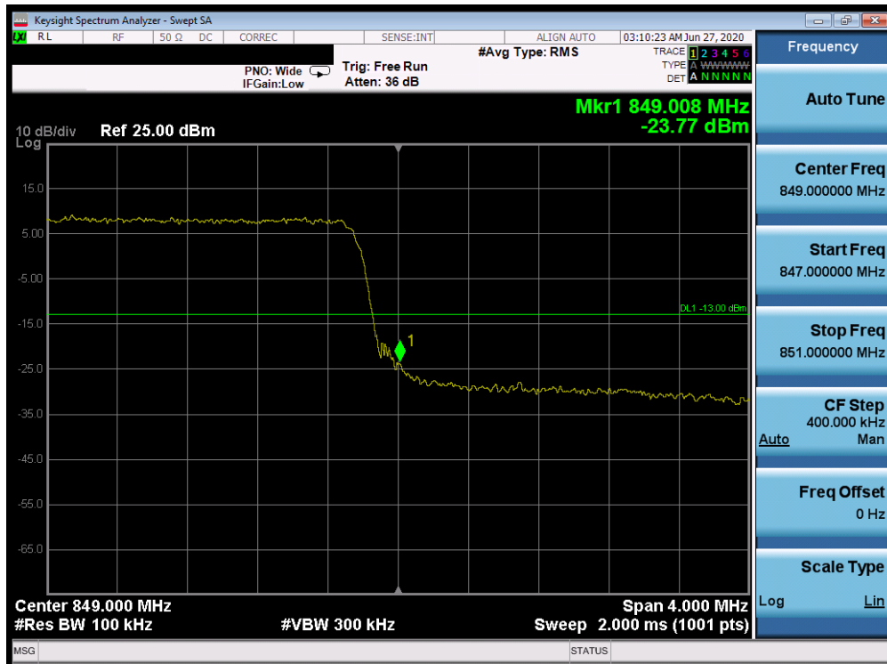
Plot 7-407. Upper Band Edge Plot (Band 26/5 - 5.0MHz QPSK - Full RB Configuration)
