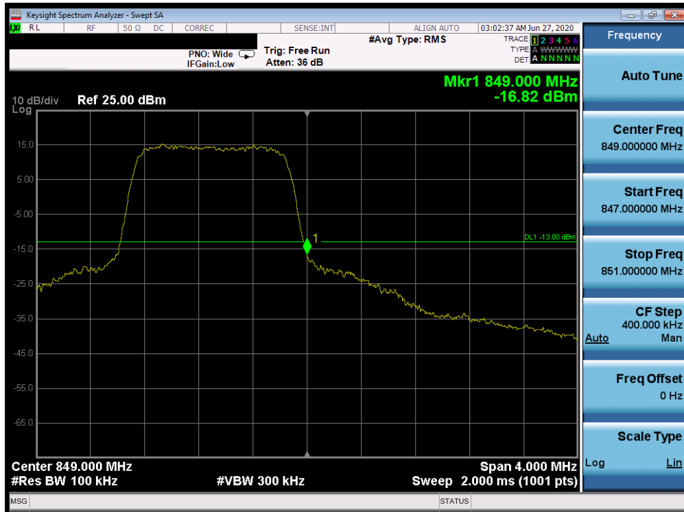
Plot 7-403. Upper Band Edge Plot (Band 26/5 - 1.4MHz QPSK - Full RB Configuration)
