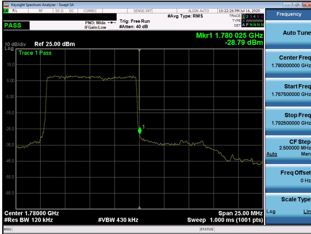
Plot 7-474. Upper Band Edge Plot (n66 - 10MHz DFT-s-OFDM-QPSK - Full RB Configuration)
