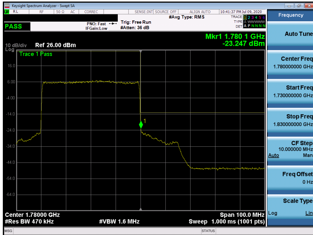
Plot 7-466. Upper Band Edge Plot (n66 - 40MHz DFT-s-OFDM-QPSK - Full RB Configuration)
