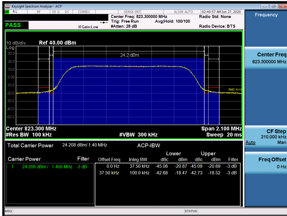
Plot 7-36. Channel Edge Plot (LTE Band 26 - 1.4MHz QPSK - High Channel)
