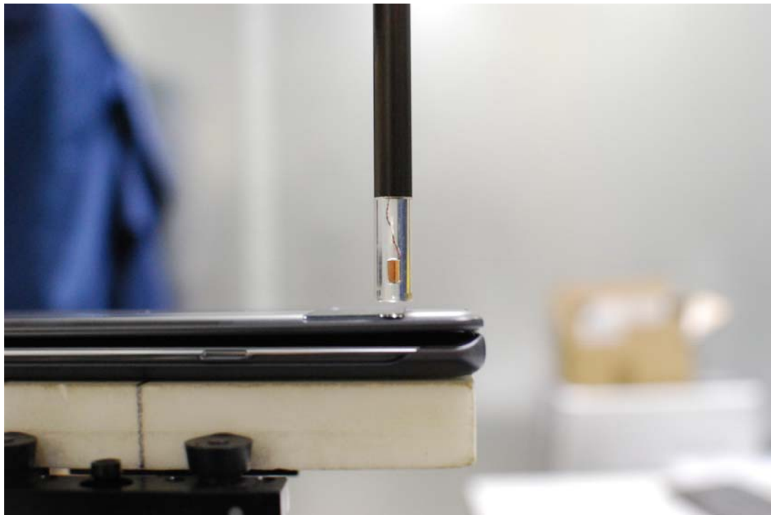
Figure 16-4 Test Setup for Wireless Device – Dual Display Closed
