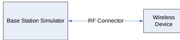
Figure 9-4 Power Measurement Setup
