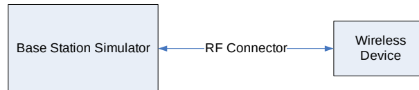
Figure 9-2 Power Measurement Setup
