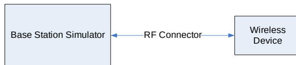
Figure 9-3 Power Measurement Setup
