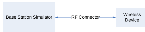
Figure 9-4 Power Measurement Setup
