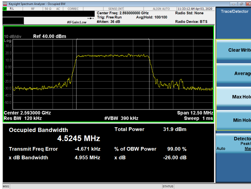
Plot 7-99. Occupied Bandwidth Plot (Band 41 - 5.0MHz 64-QAM - Full RB Configuration)
