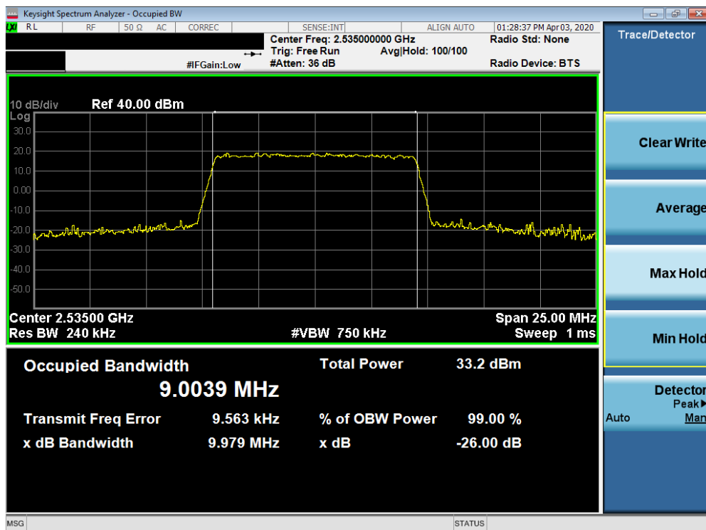
Plot 7-88. Occupied Bandwidth Plot (Band 7 - 10.0MHz QPSK - Full RB Configuration)
