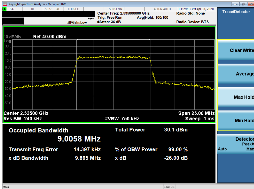
Plot 7-90. Occupied Bandwidth Plot (Band 7 - 10.0MHz 64-QAM - Full RB Configuration)
