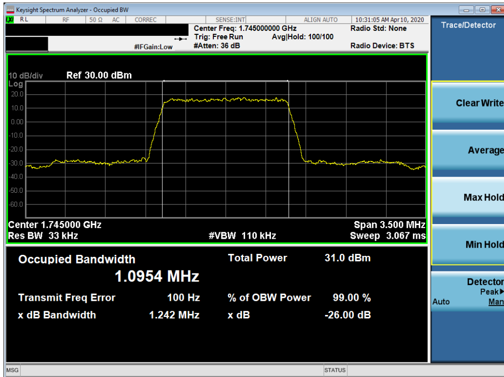
Plot 7-45. Occupied Bandwidth Plot (Band 66/4 - 1.4MHz 64-QAM - Full RB Configuration)
