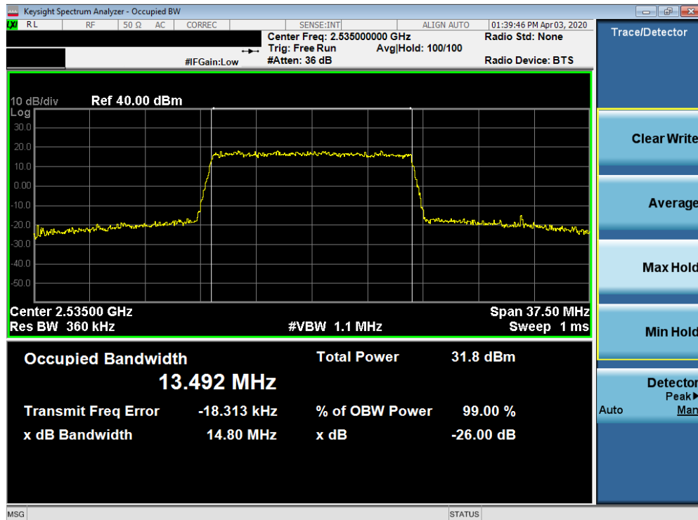
Plot 7-92. Occupied Bandwidth Plot (Band 7 - 15.0MHz 16-QAM - Full RB Configuration)
