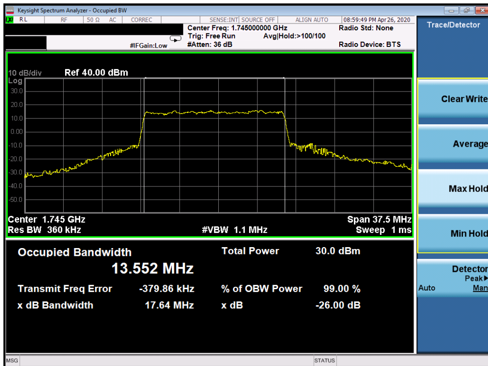
Plot 7-162. Occupied Bandwidth Plot (5G sub6 n66 - 15.0MHz 64-QAM - Full RB Configuration)
