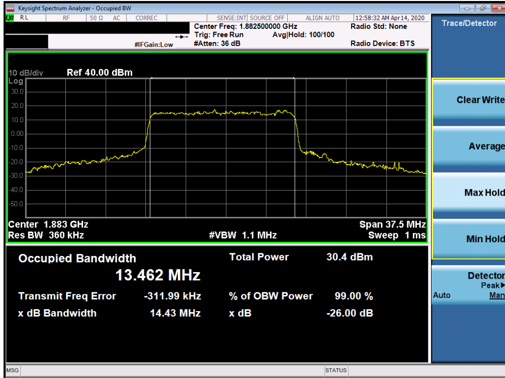
Plot 7-181. Occupied Bandwidth Plot (5G sub6 n25/2 - 15.0MHz 16-QAM - Full RB Configuration)
