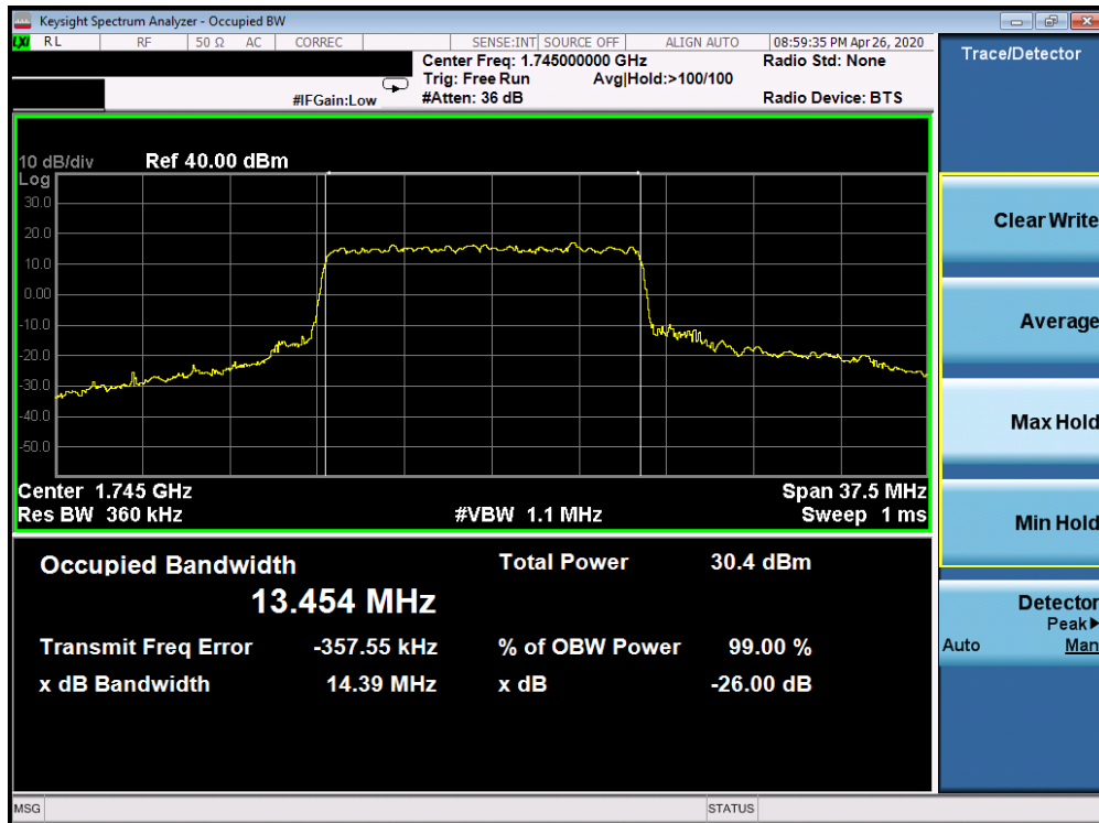
Plot 7-161. Occupied Bandwidth Plot (5G sub6 n66 - 15.0MHz 16-QAM - Full RB Configuration)
