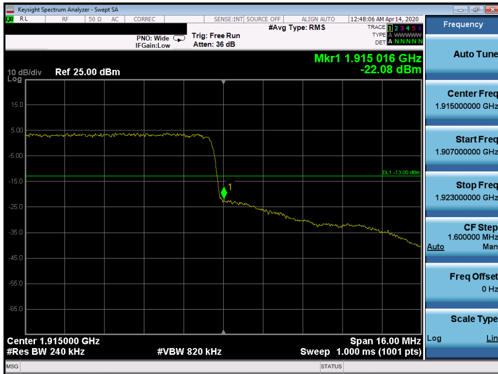
Plot 7-530. Upper 5G sub6 Band Edge Plot (5G sub6 n25 - 20.0MHz QPSK - Full RB Configuration)
