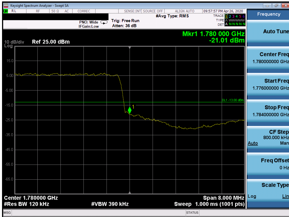
Plot 7-498. Upper 5G sub6 Band Edge Plot (5G sub6 n66 - 10.0MHz QPSK - Full RB Configuration)
