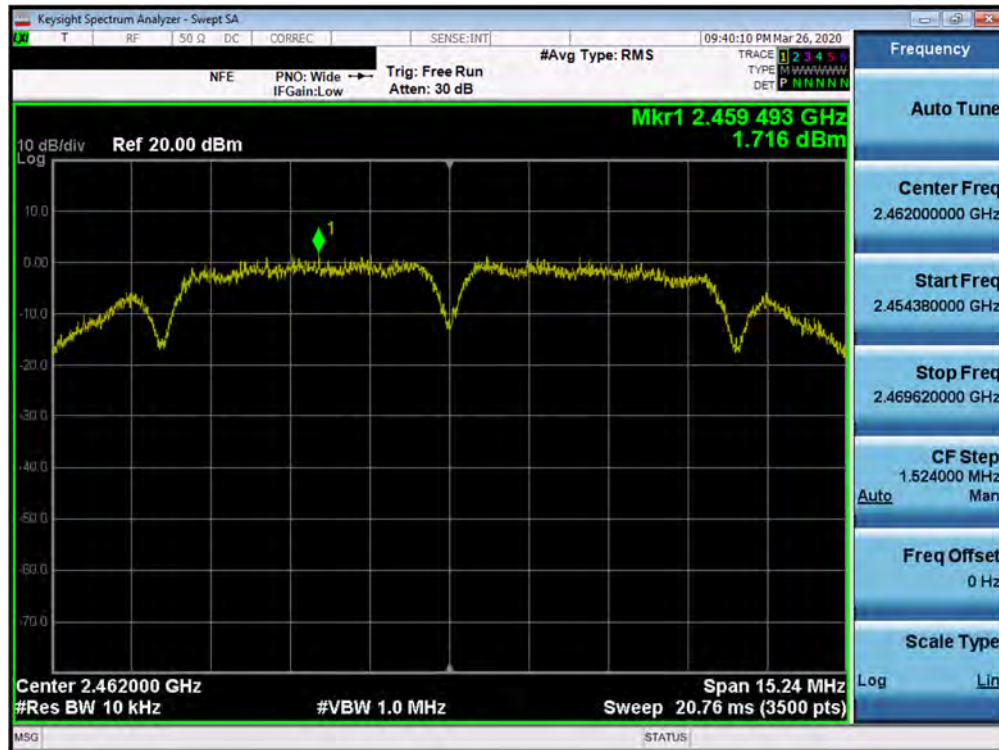
Plot 7-30. Power Spectral Density Plot SISO ANT2 (802.11b – Ch. 11)
