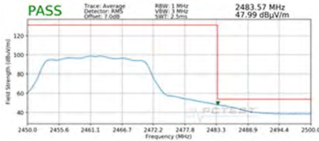
Plot 7-97. Radiated Restricted Band Edge Measurement MIMO with WCP (Average)
