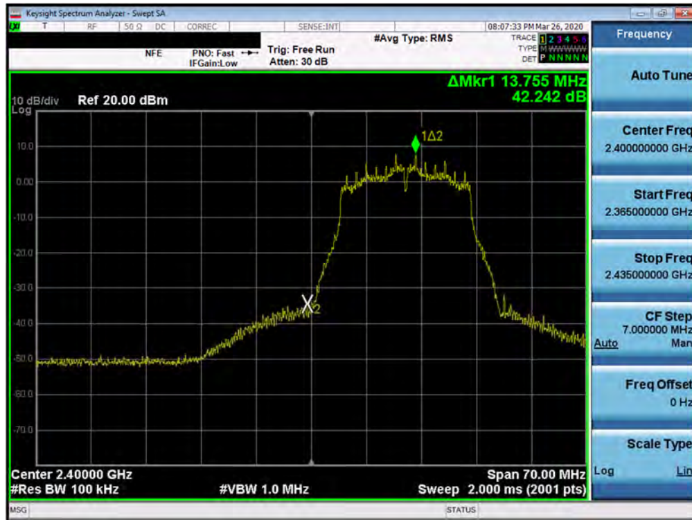
Plot 7-39. Band Edge Plot SISO ANT1 (802.11g- Ch. 1)
