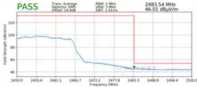
Plot 7-77. Radiated Restricted Upper Band Edge Measurement SISO ANT1 (Average)
