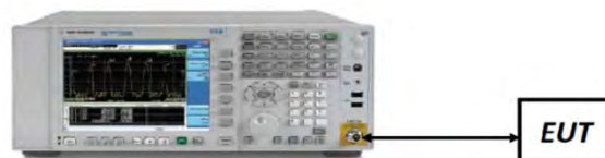
Figure 7-5. Test Instrument & Measurement Setup
