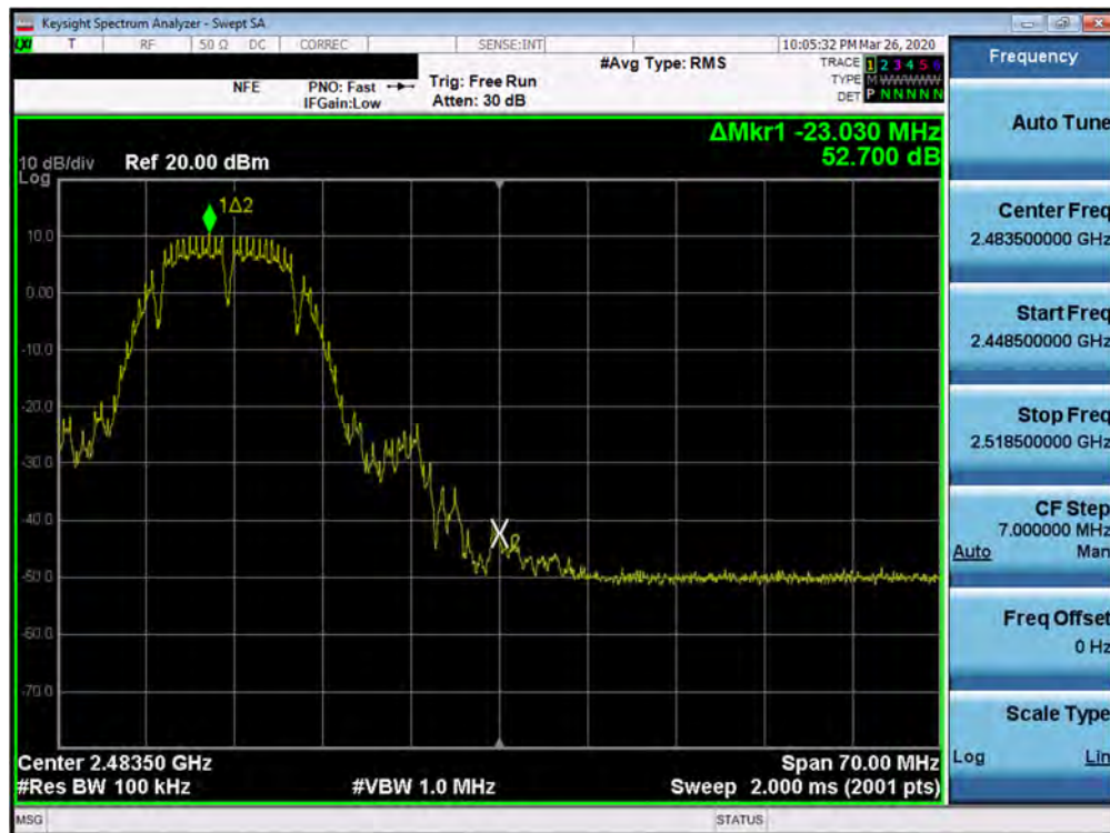
Plot 7-44. Band Edge Plot SISO ANT2 (802.11b – Ch. 11)
