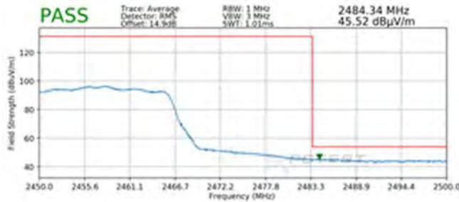
Plot 7-85. Radiated Restricted Upper Band Edge Measurement SISO ANT2 (Average)
