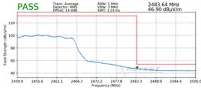
Plot 7-93. Radiated Restricted Upper Band Edge Measurement MIMO (Average)
