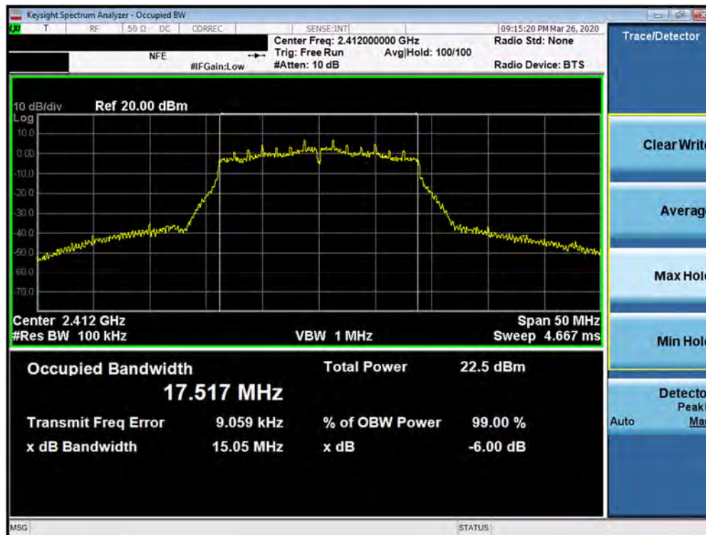
Plot 7-16. 6dB Bandwidth Plot SISO ANT1 (802.11n (2.4GHz) – Ch. 1)
