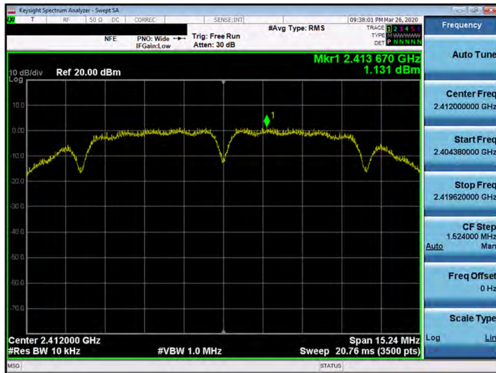
Plot 7-28. Power Spectral Density Plot SISO ANT2 (802.11b – Ch. 1)
