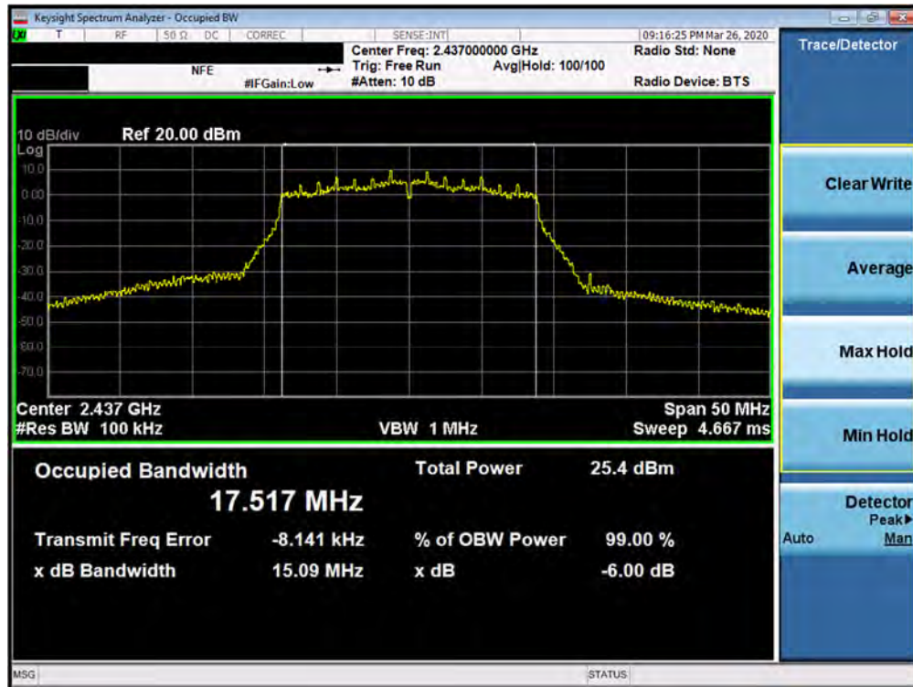
Plot 7-17. 6dB Bandwidth Plot SISO ANT1 (802.11n (2.4GHz) – Ch. 6)
