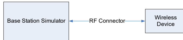
Figure 9-3 Power Measurement Setup
