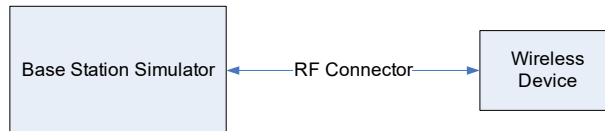
Figure 9-2 Power Measurement Setup
