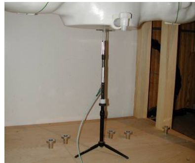
Figure 10-2 System Verification Setup Photo
