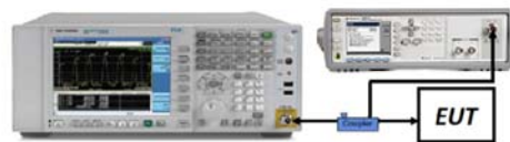
Figure 7-2. Test Instrument & Measurement Setup
