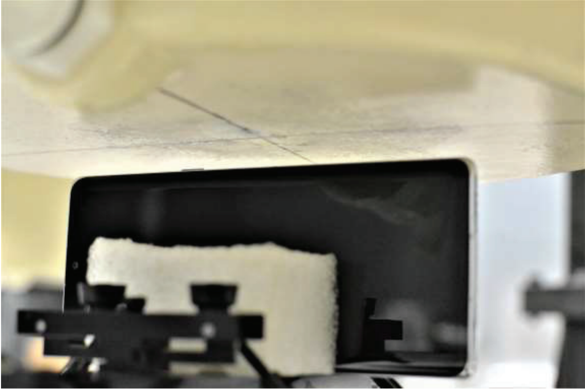
Test Setup Photo 6 – Right Edge SAR at 10 mm
