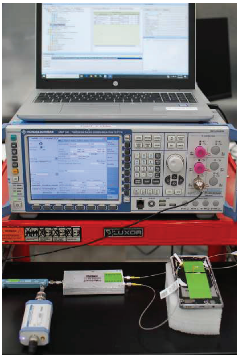
Test Setup Photo 2 – Conducted Test Setup (Figure 6-1b)
