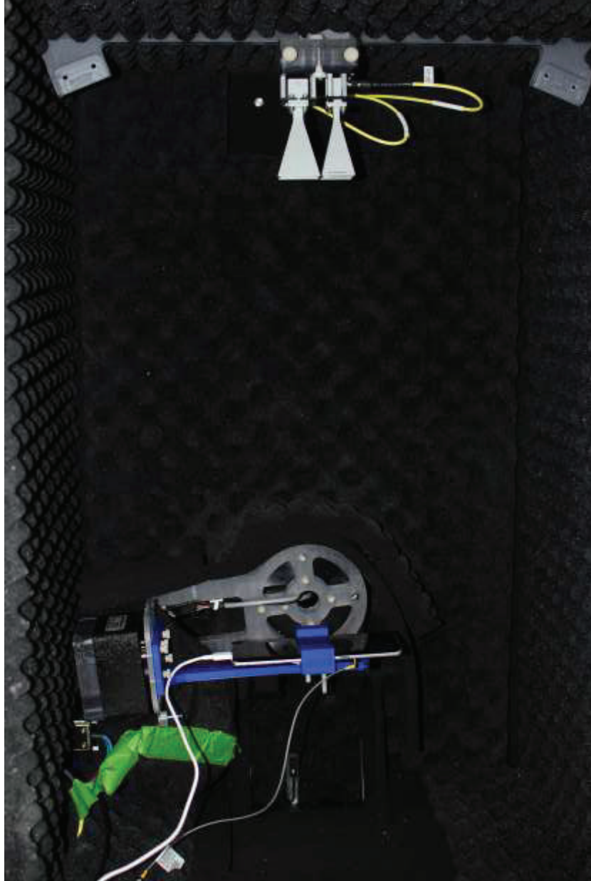
Test Setup Photo 8 – Radiated Power Measurement Setup (Figure 7-1)
