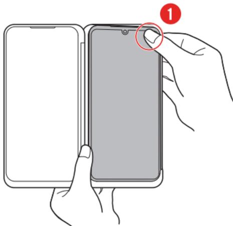
4. Press the part **2** of the phone to fully engage the Dual Screen with the phone.
