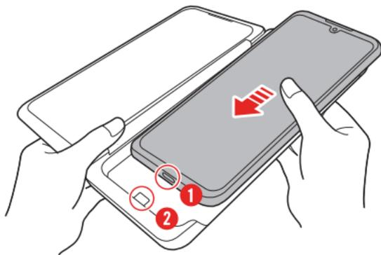
3. Press the part **1** of the phone with your finger to engage the edge of phone with that of the Dual Screen.
