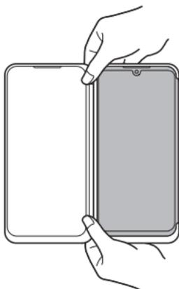
2. Press the **1** part of the Dual Screen with your finger while simultaneously pushing the back of the phone with your other finger to pull the edge of the phone out of the Dual Screen.
