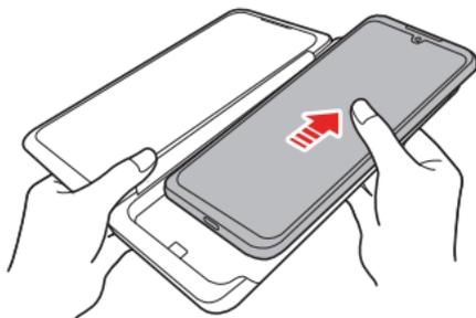
**WARNING!** Do not lift the phone from the Dual Screen at an excessive angle as shown below.
