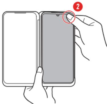
4. Hold the Dual Screen with both hands and slide the phone in the direction of the arrow to remove it. Be careful not to twist the phone left or right or push it up at an excessive angle.
