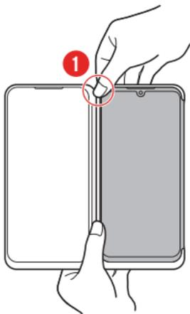
3. Pull the **2** part of the phone out of the Dual Screen following the same directions from the previous step.
