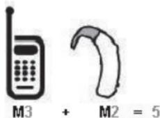
In the above example, if a hearing aid meets the M2 level rating and the wireless device meets the M3 level rating, the sum of the two values equal M5. This should provide the hearing aid user with "normal usage" while using their hearing aid with the particular wireless device. "Normal usage" in this context is defined as a signal quality that's acceptable for normal operation.
