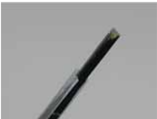
Figure 6. EX3DV4 E-field Probe
