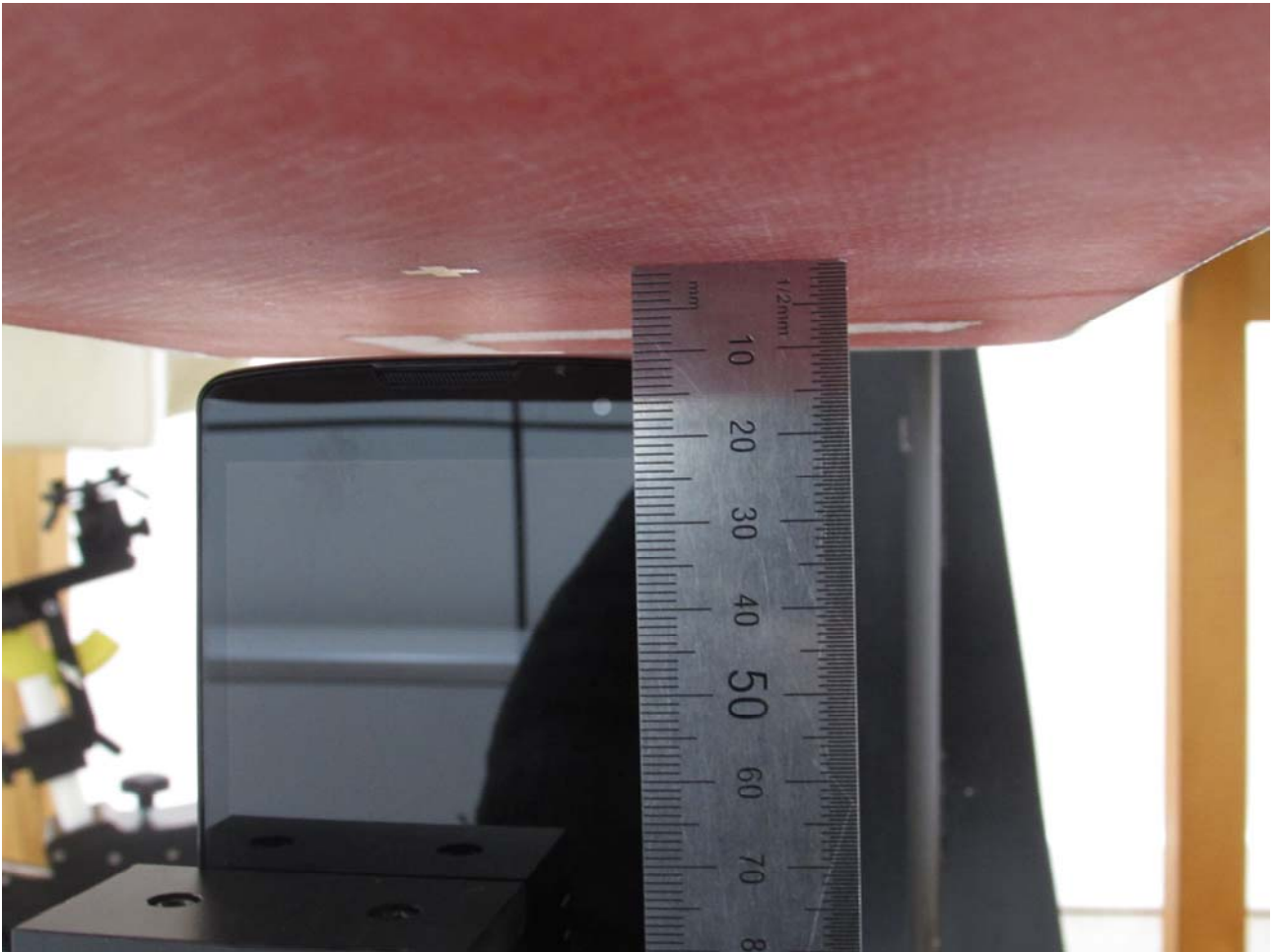
[Distance of 1.0 cm from the EUT]
