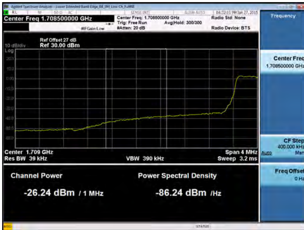
BAND 4. Lower Extended Band Edge Plot (3M BW Ch.19965 QPSK_RB15_0) -3
