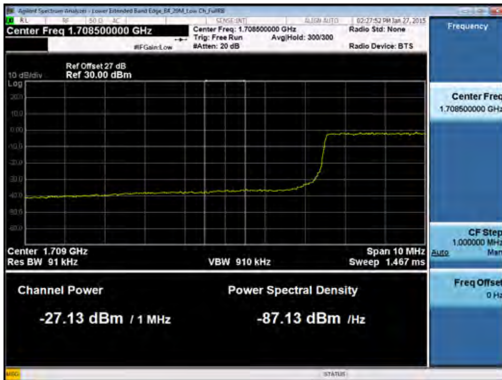
BAND 4. Lower Extended Band Edge Plot (20M BW Ch.20050 QPSK_RB100_0) -3
