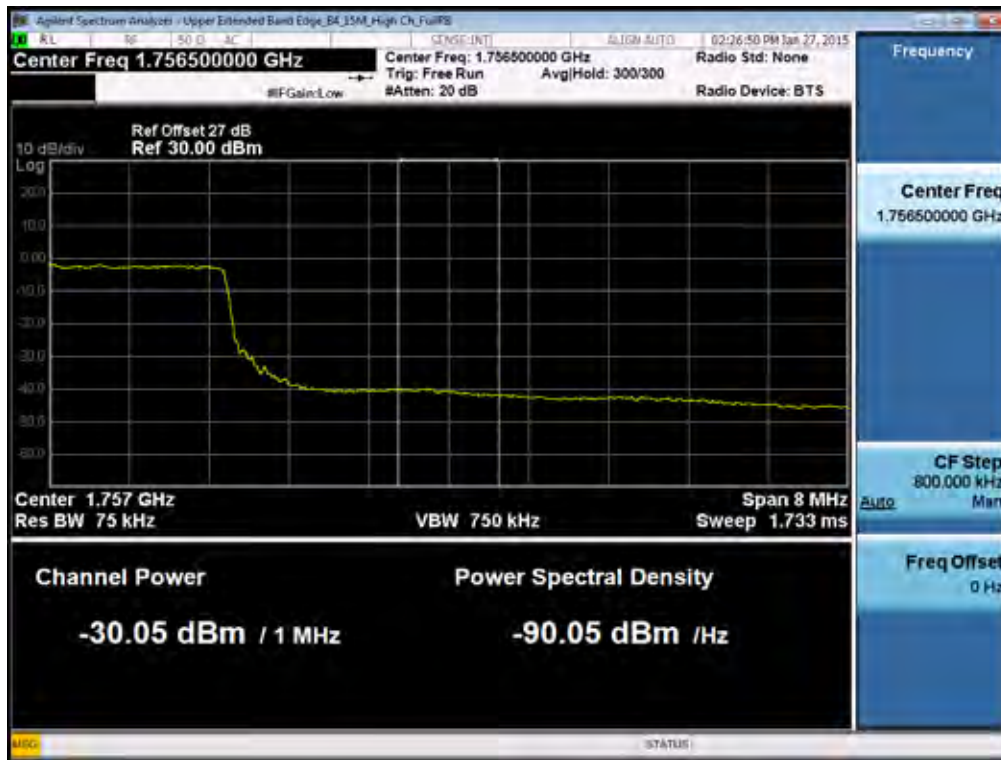
BAND 4. Upper Extended Band Edge Plot (15M BW Ch.20325 QPSK_RB75) -3
