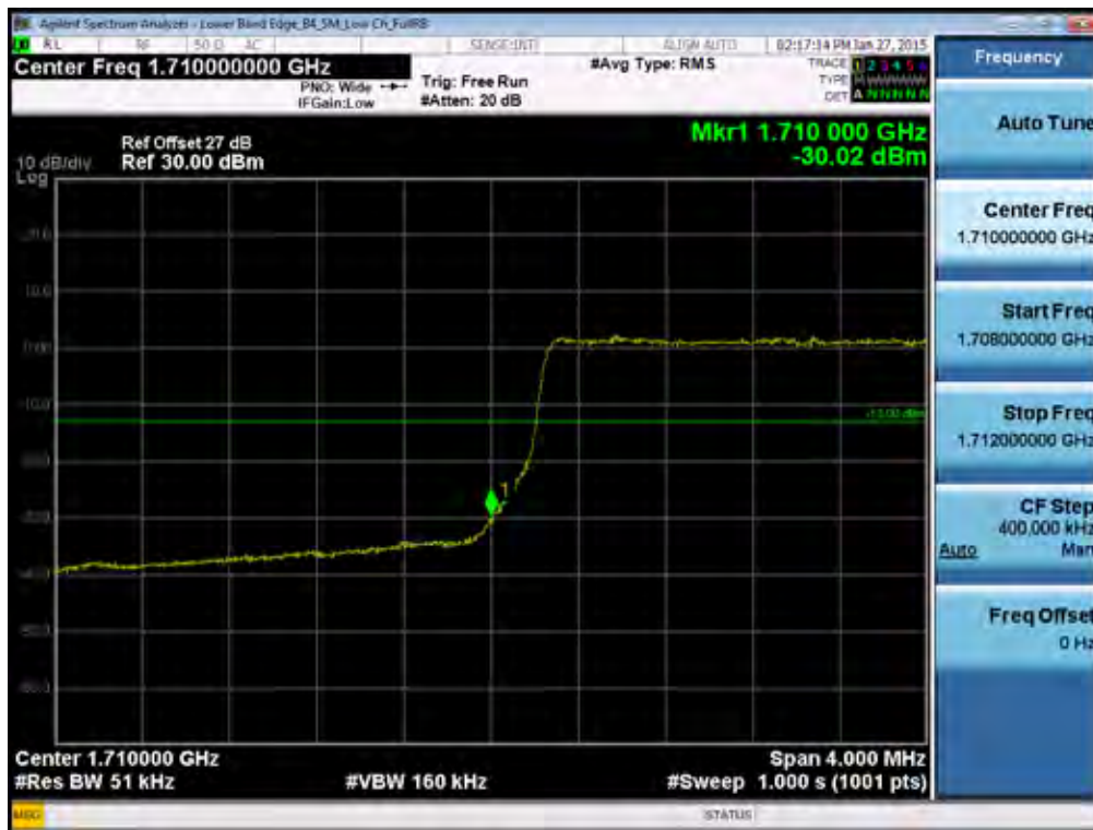
BAND 4. Lower Band Edge Plot (5M BW Ch.19975 QPSK RB 25) -2
