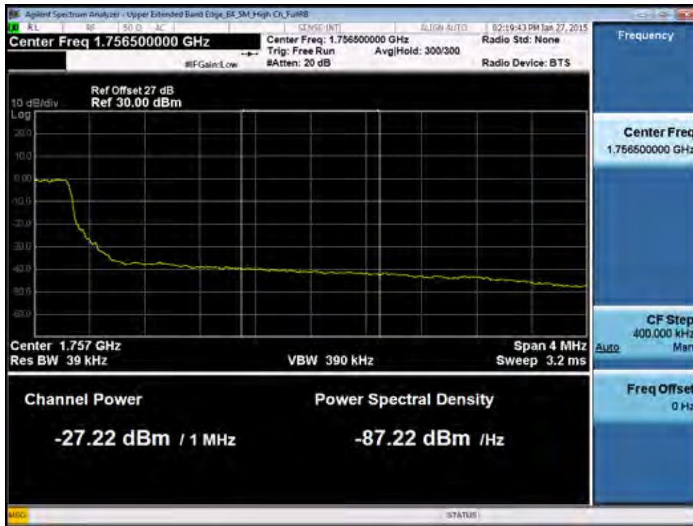
BAND 4. Upper Extended Band Edge Plot (5M BW Ch.20375 QPSK_RB25) -3
