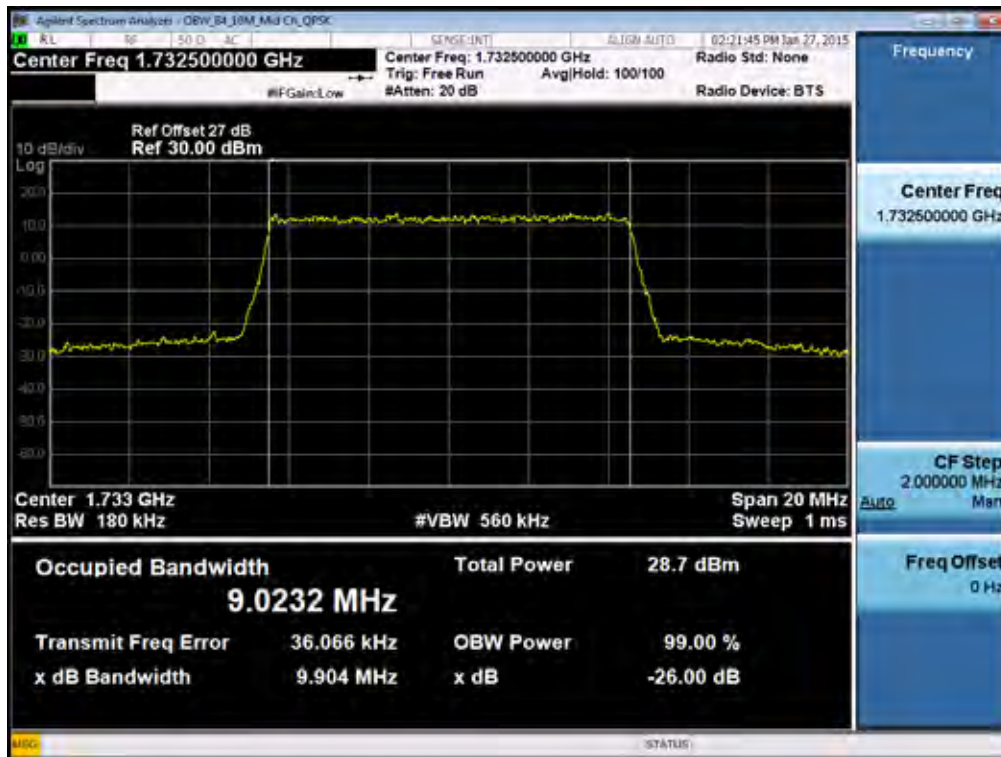
BAND 4. Occupied Bandwidth Plot (10M BW Ch.20175 QPSK RB 50)
