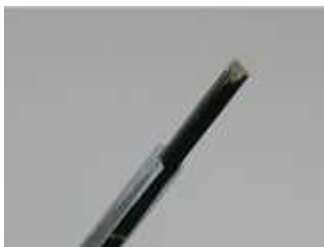
Figure 6. EX3DV4 E-field Probe
