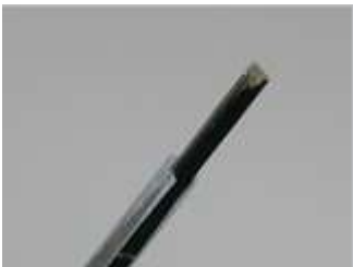
Figure 6. EX3DV4 E-field Probe
