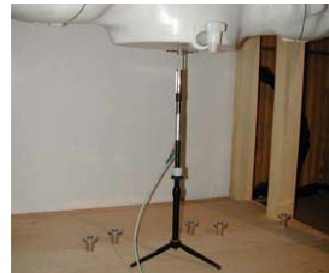
Figure 11.1 Dipole Verification Test Setup Diagram & Photo
