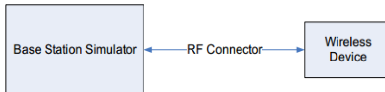
Figure 10.2 Power Measurement Setup
