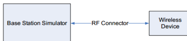
Figure 10.1 Power Measurement Setup
