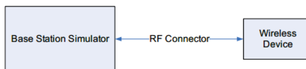
Figure 10.1 Power Measurement Setup
