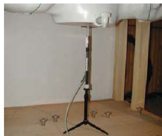
Figure 11.1 Dipole Verification Test Setup Diagram & Photo
