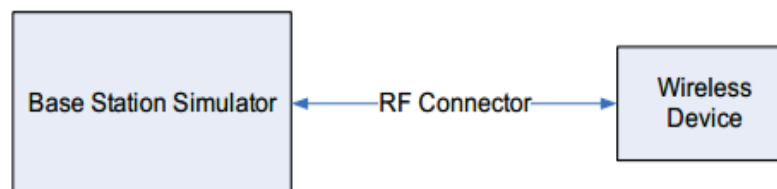
Figure 10.2 Power Measurement Setup
