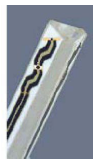
Figure 3.3 Probe Thick-Film Technique
