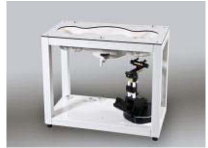
Figure 3.6 SAM Twin Phantom
