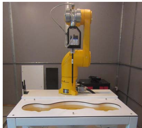
Figure 2.2 DASY5 Test System
