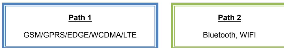
Figure 13.1 Simultaneous Transmission Paths
