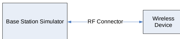
Figure 9-2 Power Measurement Setup
