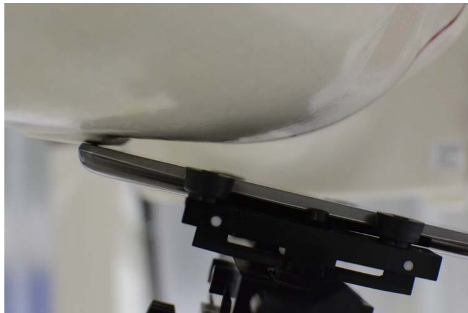
SAR Test Setup Photo 2 – Right Tilt
