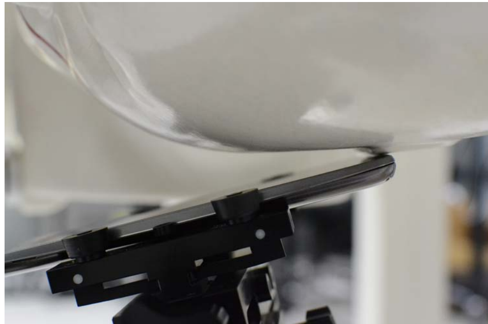
SAR Test Setup Photo 4 – Left Tilt
