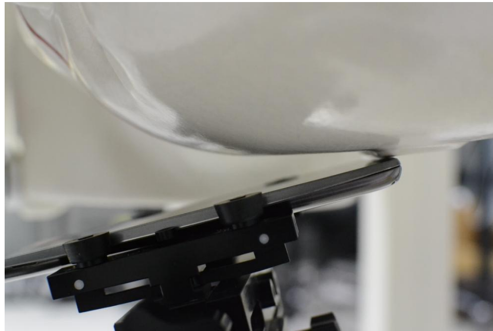
SAR Test Setup Photo 6 – Left Tilt
