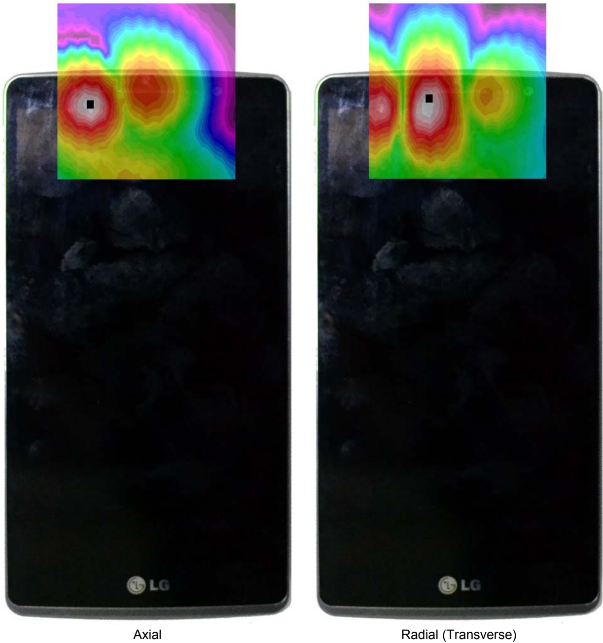
Figure 12-3 T-Coil Scan Overlay Magnetic Field Distributions
