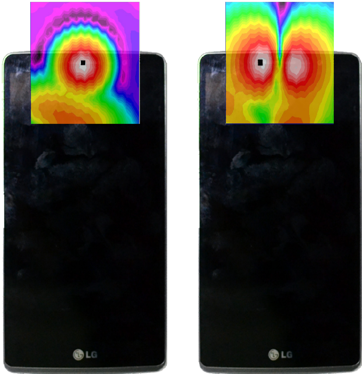
Figure 12-7 T-Coil Scan Overlay Magnetic Field Distributions
