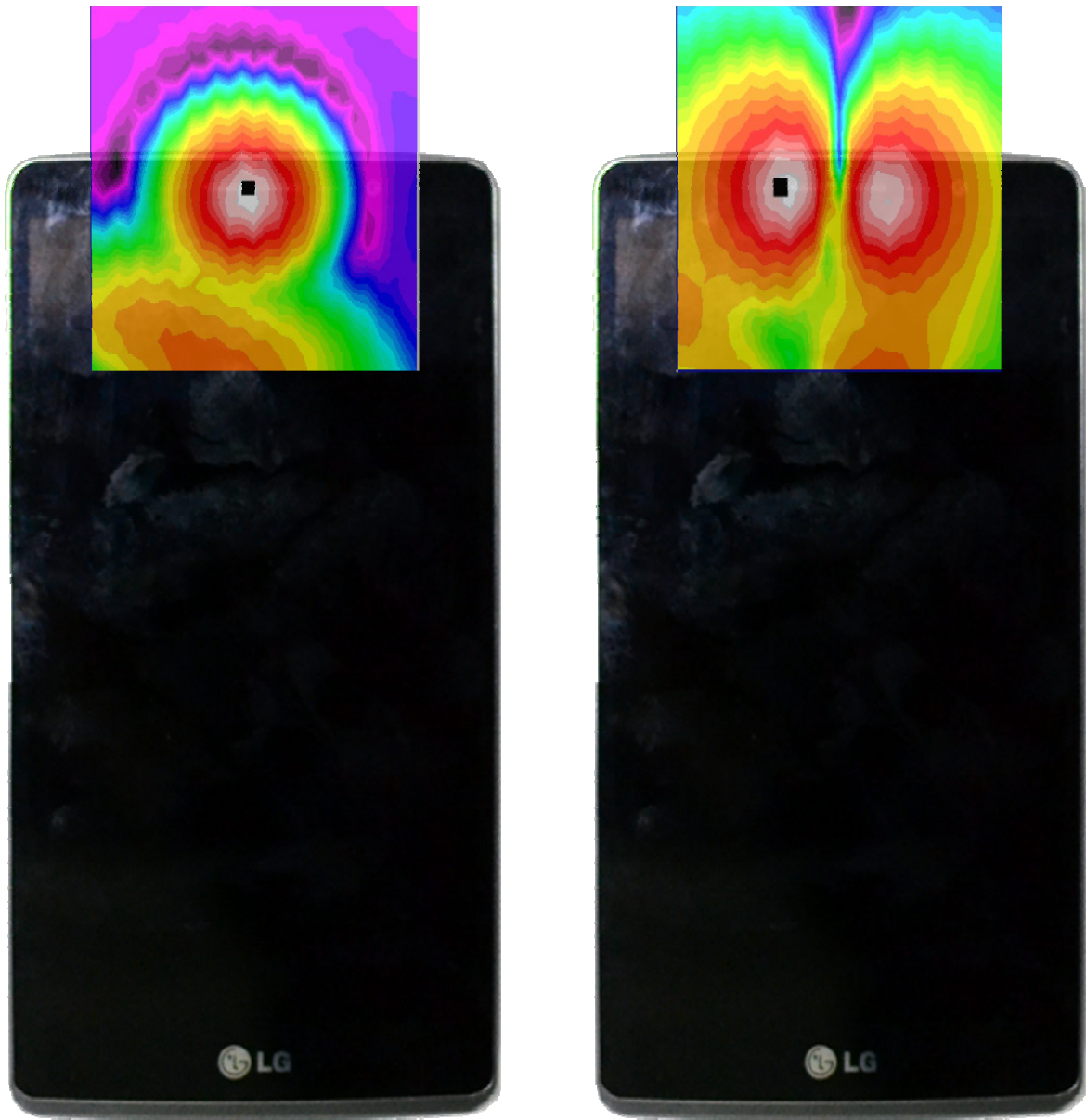
Figure 12-7 T-Coil Scan Overlay Magnetic Field Distributions
