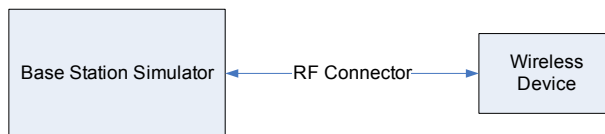
Figure 9-1 Power Measurement Setup
