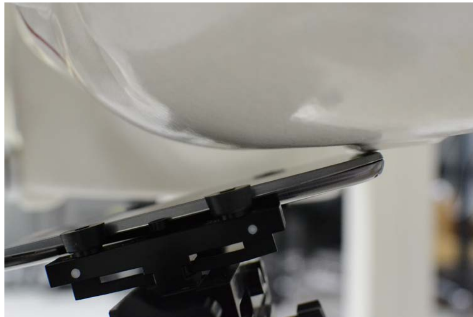
SAR Test Setup Photo 4 – Left Tilt
