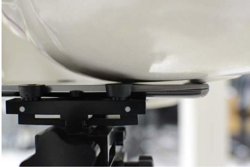
SAR Test Setup Photo 3 – Left Cheek
