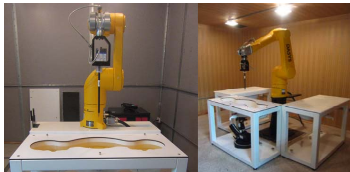
Figure 2.2 DASY5 Test System
