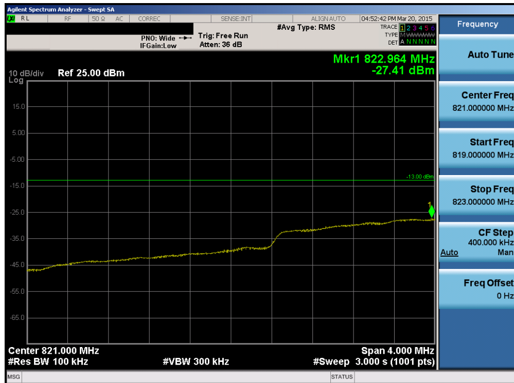
Plot 6-113. Lower Extended Band Edge Plot (Band 5 – 3.0MHz QPSK – RB Size 15)
