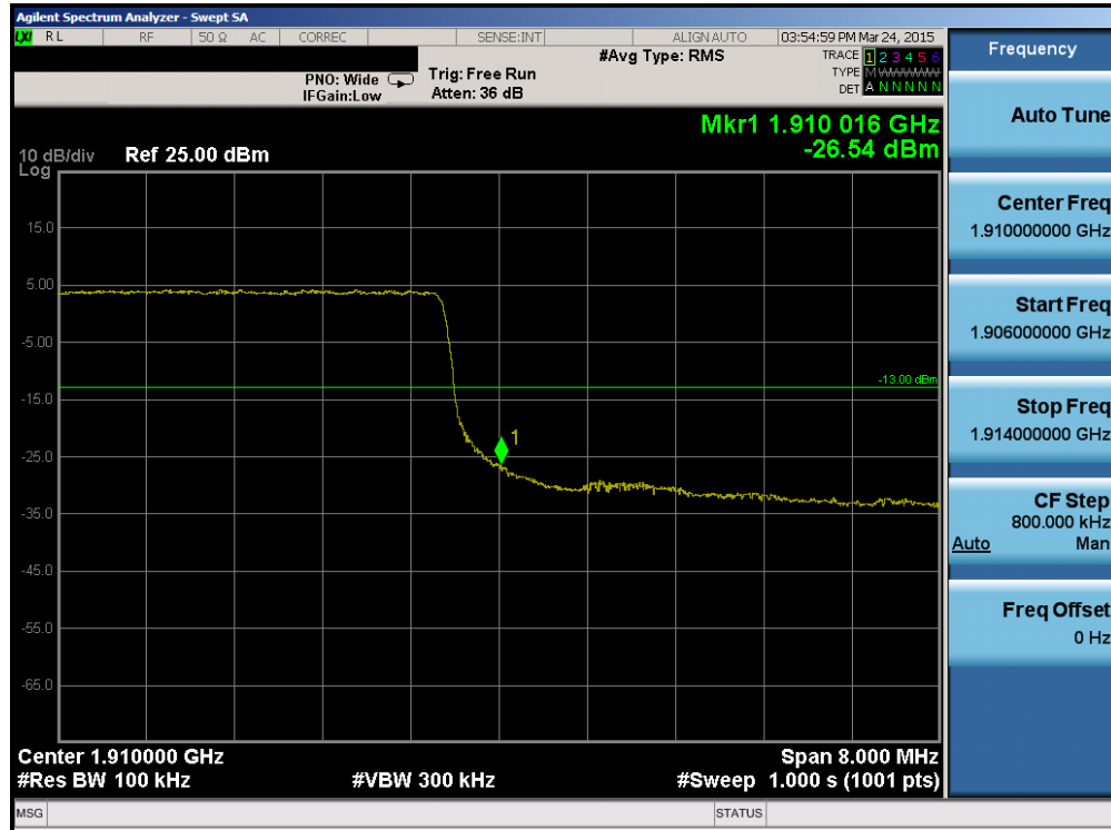
Plot 6-160. Upper Band Edge Plot (Band 2 – 10.0MHz QPSK – RB Size 50)
