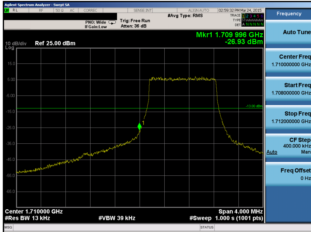
Plot 6-122. Lower Band Edge Plot (Band 4 – 1.4MHz QPSK – RB Size 6)
