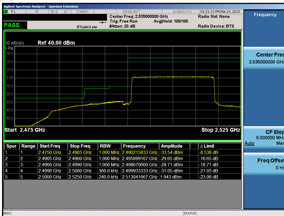
Plot 6-176. Lower ACP Plot (Band 7 – 20.0MHz QPSK – RB Size 100)
