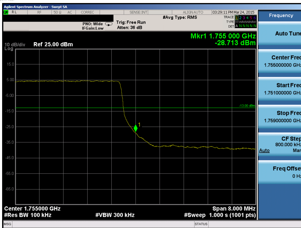
Plot 6-136. Upper Band Edge Plot (Band 4 – 10.0MHz QPSK – RB Size 50)
