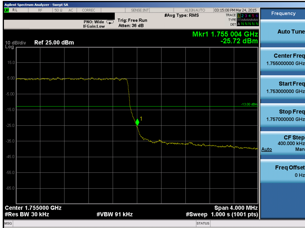
Plot 6-128. Upper Band Edge Plot (Band 4 – 3.0MHz QPSK – RB Size 15)
