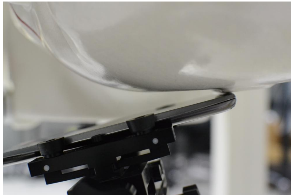
SAR Test Setup Photo 4 – Left Tilt
