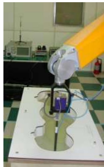
Figure 3. Photograph of the probe and the Phantom
