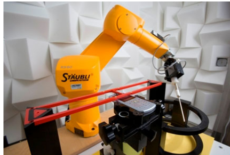
Figure 4-3 SPEAG Robotic System
