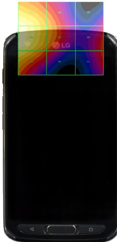
Figure 17-4 E-Field WD Scan overlay
