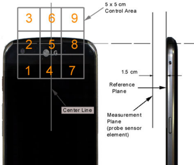
Figure 17-3 5x5 Scan grid above WD
