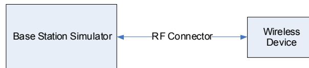
Figure 9-2 Power Measurement Setup
