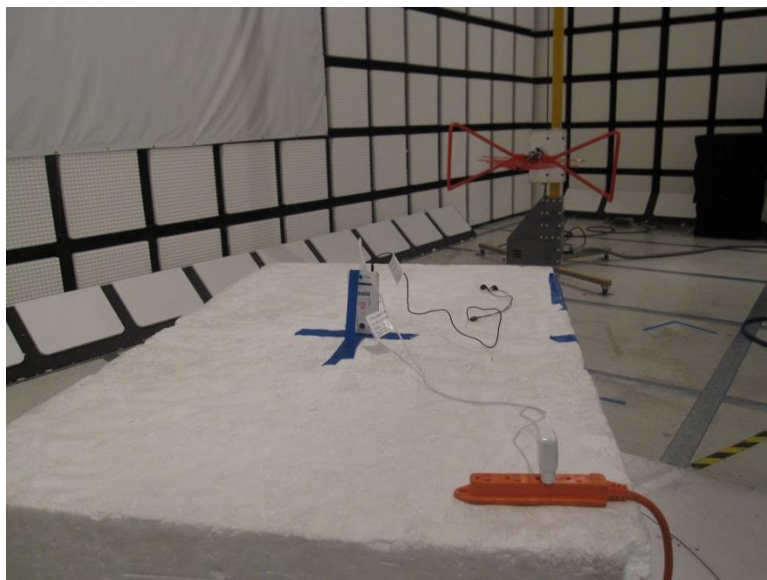
RADIATED BACK PHOTO (BELOW 1 GHz)
