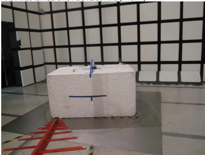
RADIATED EMISSIONS ABOVE 30 MHz (FRONT)
