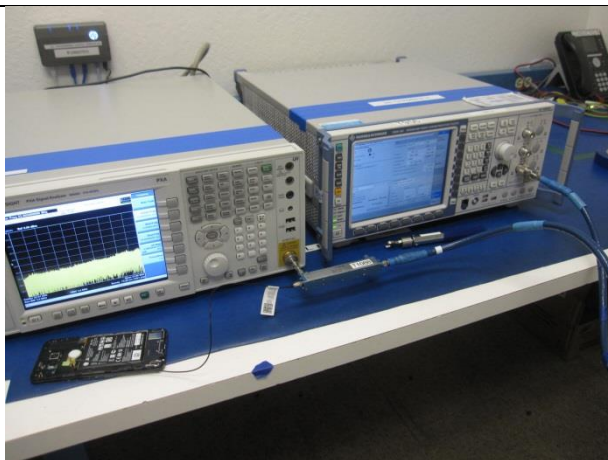
ANTENNA PORT CONDUCTED PHOTO
